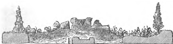
Fig. 4.—The same Road, in its third year after repair, or its last and worst state.
