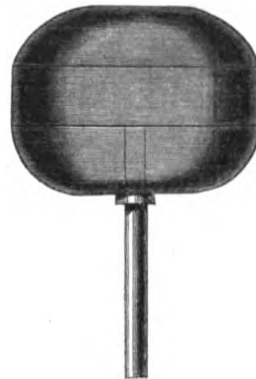
VIEW OF CARBON FILTER.
