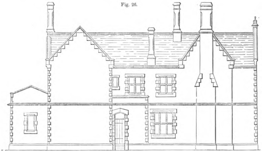
SIDE ELEVATION OF FARMHOUSE—SCALE IN PLATE XVIII.
