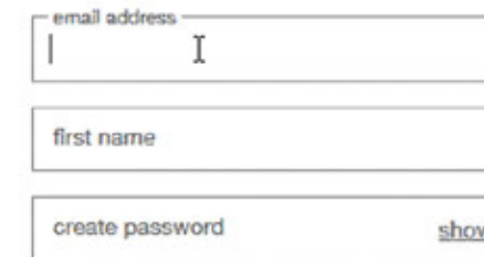
Figure 14. A newer interactive form that provides assistance to users by moving the label text from being a placeholder to hovering above the field.
