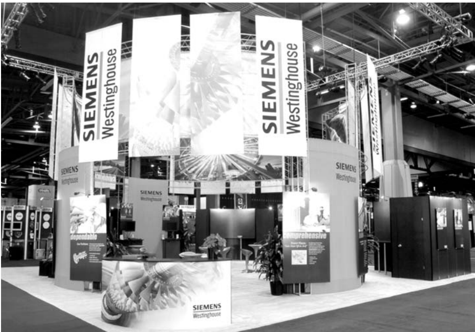
Figure 14.1 A large island exhibit created by Skyline Exhibits uses modular truss to carry colorful, lightweight fabric graphics. This creates a sense of mass and brings the company name into view from across the trade show floor.
